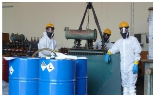
PCBs as dielectric and coolant fluids in electrical apparatus.
